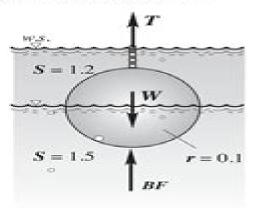
② Tension in the cable attached to the sphere to normal position
