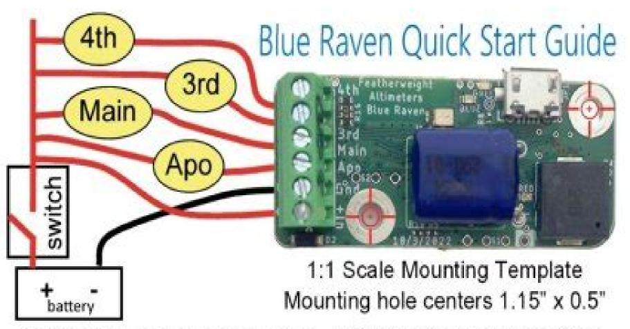
Installation: Mount any orientation. Avoid direct sun. Battery voltage between 3.6V and 16V. Output current up to 20 Amps.
