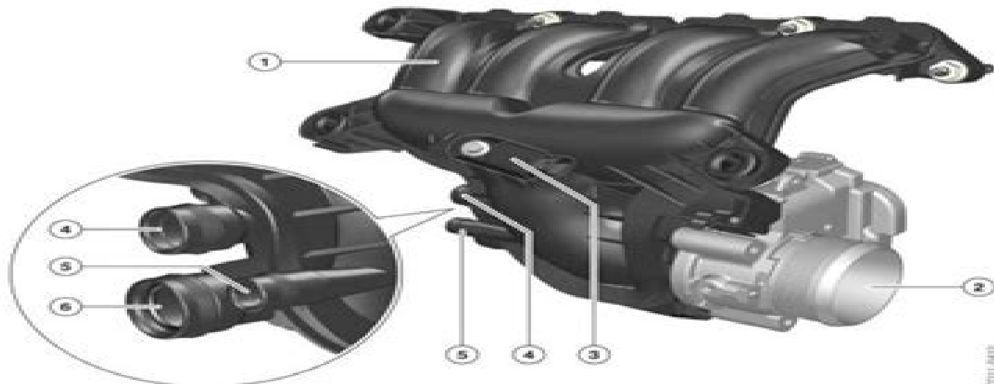
N13 engine, intake manifold with throttle valve
