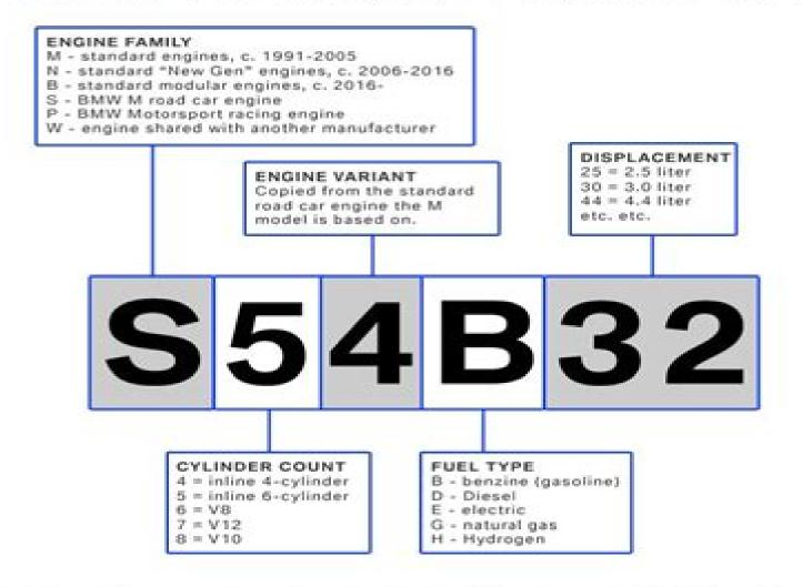
Translation: M road car engine I inline-6 | Based on M54 | Gasoline | 3.2-liter
