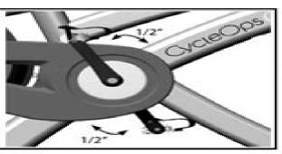
Move the crank arms back and forth. If there is more than 1/2" movement in the chain before the flywheel rotates, the chain needs to be re-adjusted.
