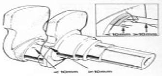
The shaft must be scrapped when cracks are longer than 10 mm outside the marked area. Isolated cracks less than 10 mm are acceptable.
