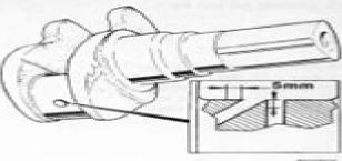
The shaft must be acrapped when cracks longer than 5 mm are adjacent to the area around the oil holes. Cracks shorter than 5 mm can be removed by grinding.
