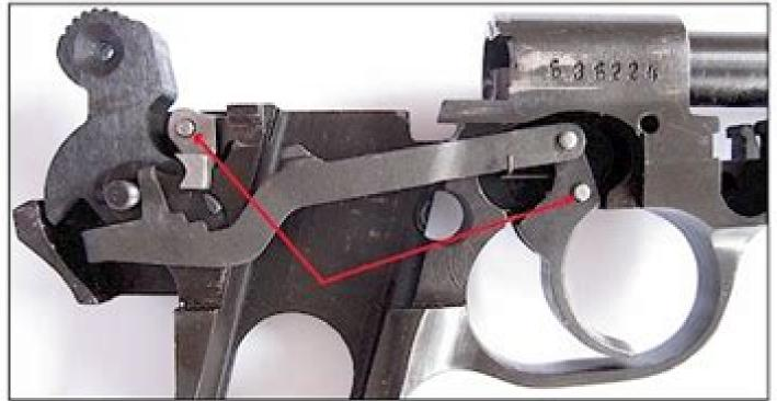
If the retaining pins of the cover plate had been (as recommended) disengaged by a short push toward the left side of the gun, after the removal of the plate all the moving parts inside the mechanism would have remained attached at the frame. The immediate reinstallation of the plate would be as fast and easy as its dismounting. This, of course, is no longer the case when the retaining pins have been pushed, from the left side of the frame.
