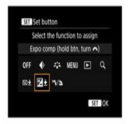
Custom controls is used to assign the SET button to allow exposure compensation to be changed.
