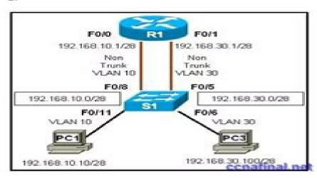
Refer to the exhibit. R1 is routing between networks 192.168.10.0/28 and 192.168.30.0/28. PC1 can ping R1 interface F0/1, but cannot ping PC3. What is causing this failure?
