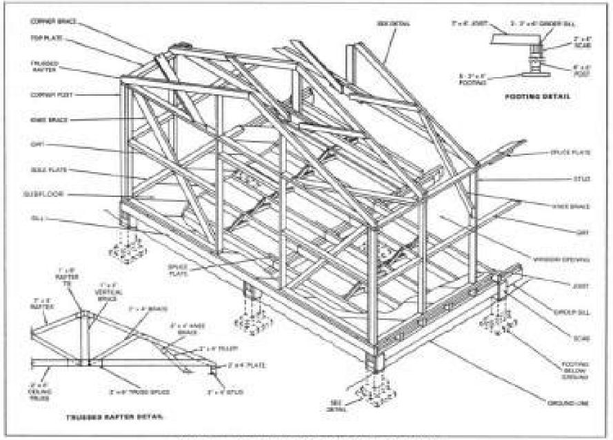
Figure 1-13. Light framing details (20-loot-wide building)
