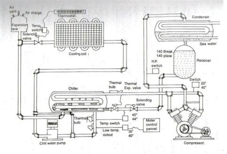
Fig. 8.1 Chilled water circulating system.
