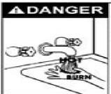
Water temperature over 125°F (52°C) can cause severe burns instantly resulting in severe injury or death.
