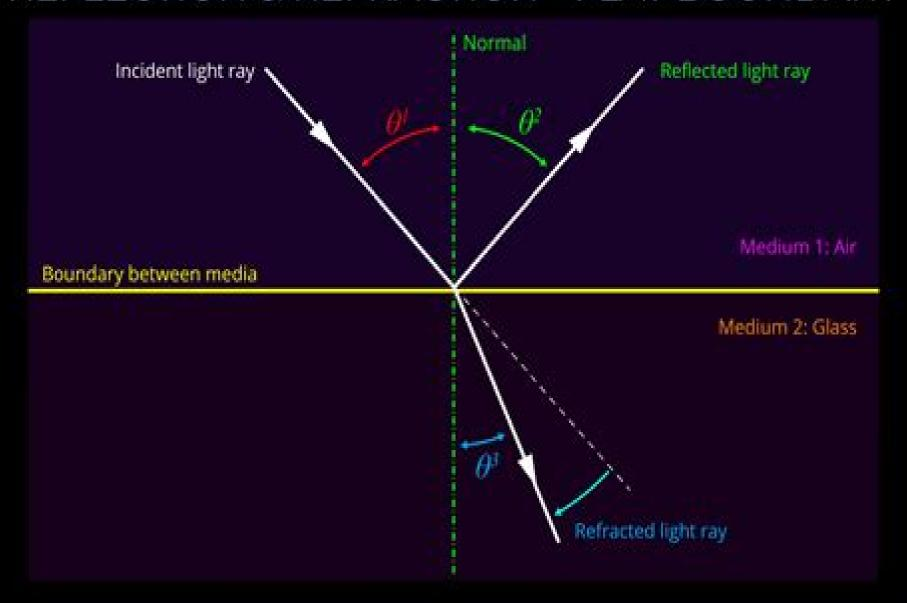
Angle of incidence  $\theta^*$  = Angle of reflection  $\theta^*$ . Angle of refraction  $\theta^*$ . The refracted light ray bends towards the normal as the light travels from air to glass.
