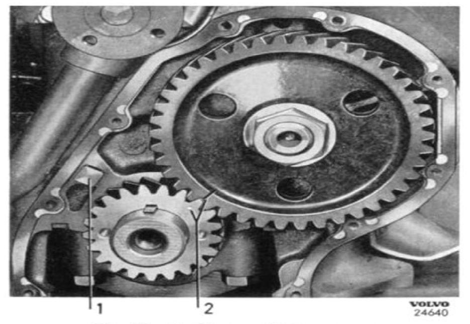
Fig. 49 Marking on timing gears
