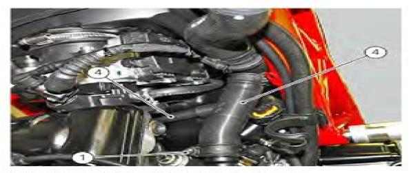
Loosen clip (5) of radiator / thermostat hose (4) to the horizontal head. Remove the hose (4).
