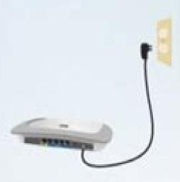
Plug the Internet cable into the yellow port in the back of your router labeled "Internet." Plug the other end into the modem.
