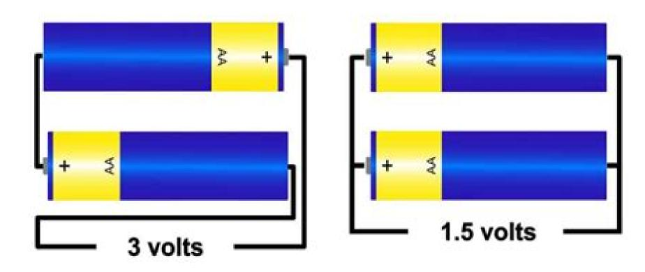
Two 1.5 volt batteries in series equals 3 volts.
