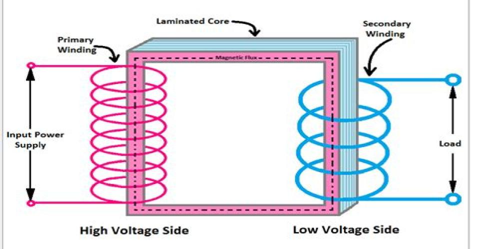
**Step Down Transformer Diagram**
