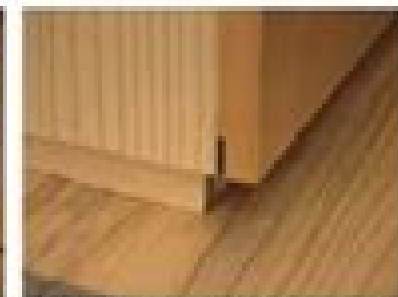
step 21 • This is a view of the front door to the side of the back panel. Use a nail gun to attach the front door to the side of the back panel.
