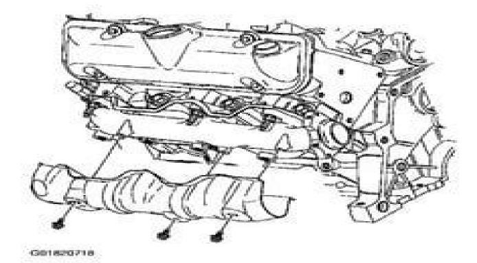
Fig. 7: Removing Exhaust Manifold Heat Shield Courtesy of GENERAL MOTORS CORP.
