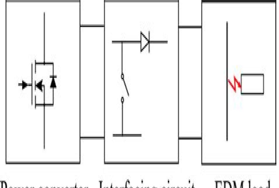
Power converter Interfacing circuit EDM load
