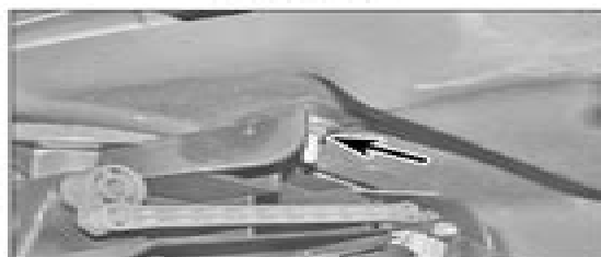
9.22d There is a mounting nut on the top right ...
