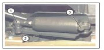
With engine off, check the clearance between the control arm (1) and the stop (2). In the brake valve "OFF" position, the control arm should be resting on the stop.
