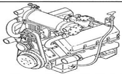
ENGINE, DIESEL, LIQUID COOLED V-TYPE, EIGHT CYLINDER, CUMMINS MODEL V903C W/CONTAINER (NSN 2815-01-399-6801)
