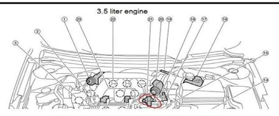
EVAP canister purge volume control solenoid valve
