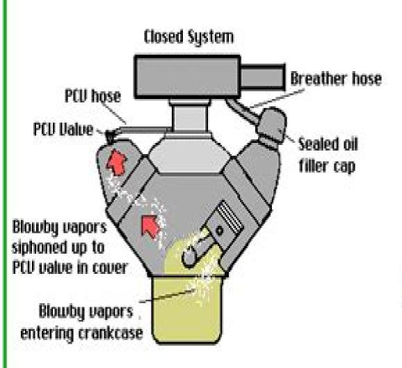
PCV Valve Minimum flow at idle/low speed
