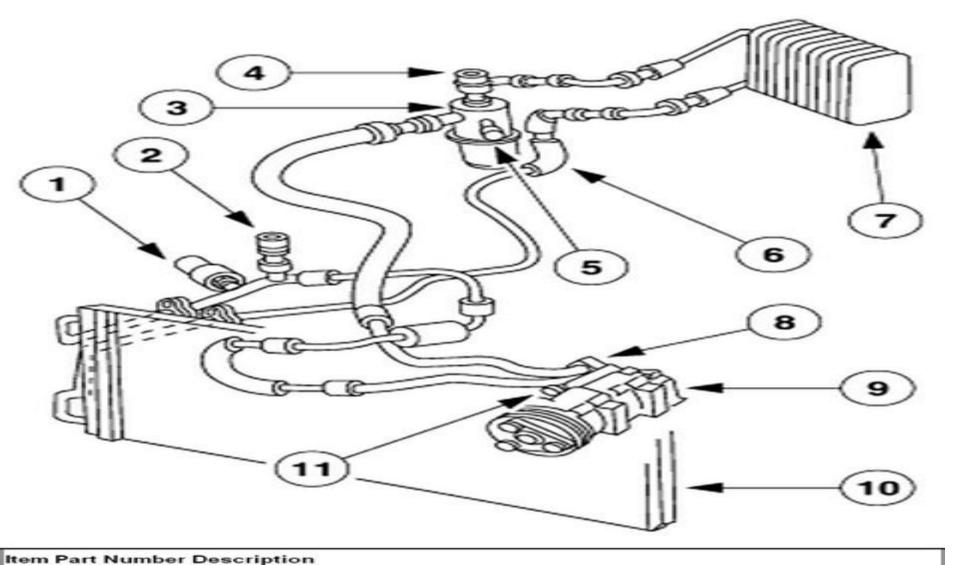
1 19D594 A/C Pressure Cut-Off Switch
