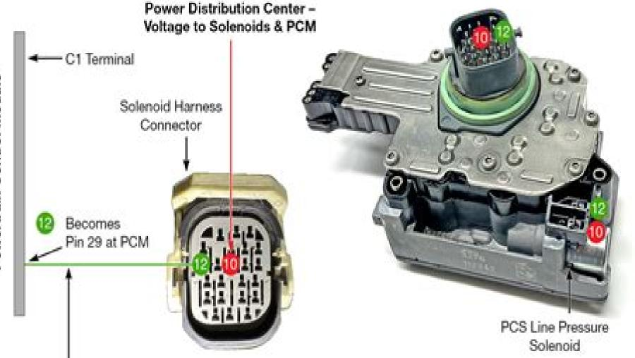
PCS Line Pressure Solenoid PWM Ground Control Circuit Check for wire breaks or green corrosion at connectors. This may also be PCM, solenoid pack or PCS line pressure solenoid fault.
