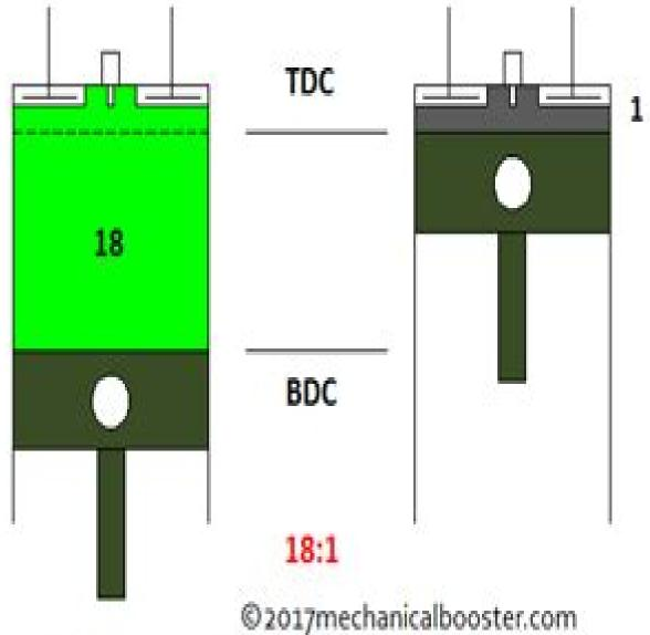
**Compression Ratio of Diesel Engine**
