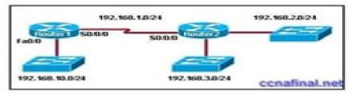
Refer to the exhibit. The network that is shown is running RIPv1. The 192.168.10.0/24 network was recently added and will only contain end users. What command or set of commands should be entered on Router1 to prevent RIPv1 updates from being sent to the end user devices on the new network while still allowing this new network to be advertised to other routers?
