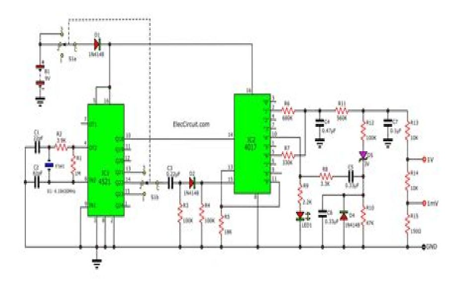
ECG simulator circuit using CD4521 and CD4017
