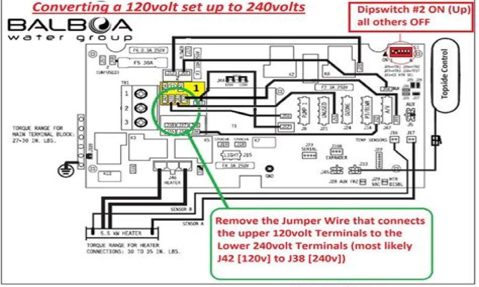
The Pump must remain on the 120volt set up as it is not 240volt compatible. Do not move J50 from J39 and J51 from J41.
