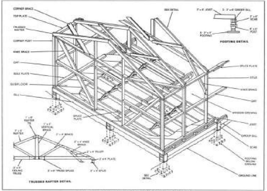
Figure 1-13. Light framing details (20-loot-wide building)
