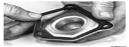
If necessary, install a new gasket in the cover.
