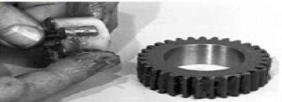
Lubricate the bearings and teeth of the idler gear with the grease specified on page 3.
