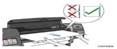
8 When the paper is correctly aligned with the blue dashed lines on the sheet paper entry platen lower the handles to hold the paper in place.
