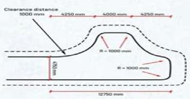
Hammerhead turning place for cars
