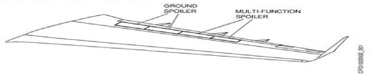
The system is computer controlled and hydraulically operated, two ground spoilers provide ground lift dumping functions. The multifunction spoilers provide roll assist, proportional lift dumping and ground lift dumping functions.
