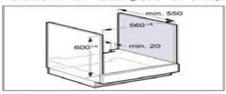
To ventilate the appliance, the intermediate floor must have a ventilation cut-out.
