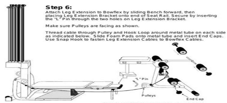
To leave Leg Extension on machine when not in use, unhook Leg Extension Cables from Bowflex Cables.
