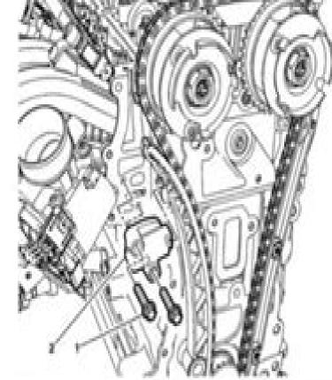
Remove the carrelast timing chain. Refer to Carolinst Timing Chain Replacement.
