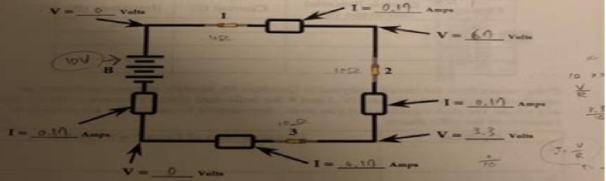
For resistors 1, 2, and 3 and for the battery (B), calculate the electric potential difference and fill in the table below.
