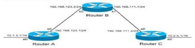
We'll assume that RIPv1 is configured correctly on all routers. Notice that our networks are no longer contiguous. Both Router A and Router C contain subnets of the 10.0.0.0 major network (10.1.0.0 and 10.2.0.0 respectively).
