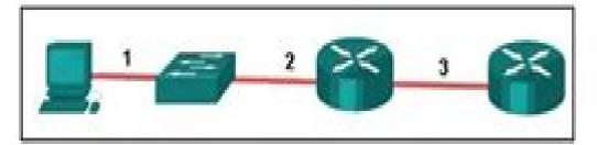
Refer to the exhibit. The PC is connected to the console port of the switch. All the other connections are made through FastEthernet links. Which types of UTP cables can be used to connect the devices ?
