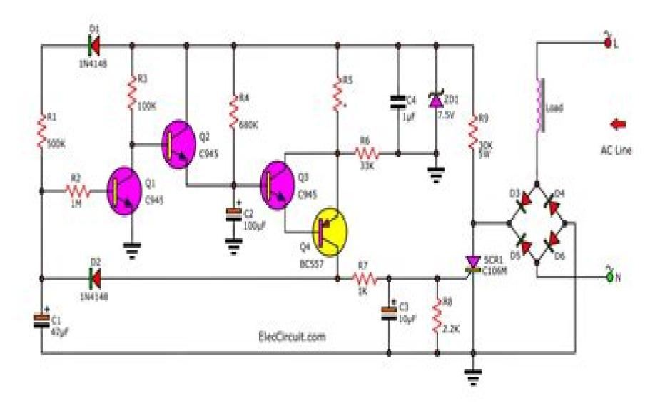
Air Compressor Time delay circuit
