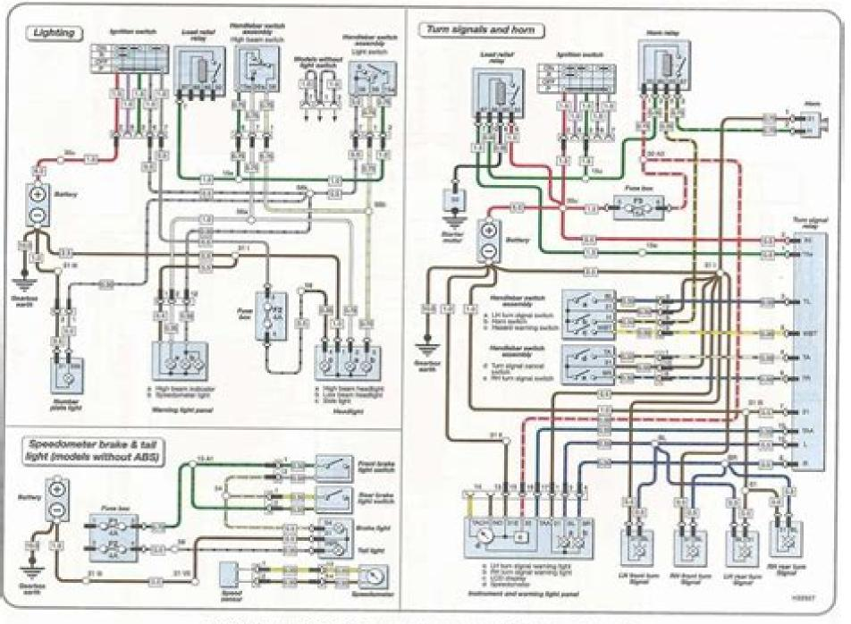
R1100 S ('01 onwards): Lighting, speedometer, brake and tall lights, turn signals and horn
