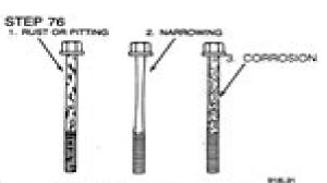
Check and replace all head boits that have rust, pitting narrowing and corrosion.
