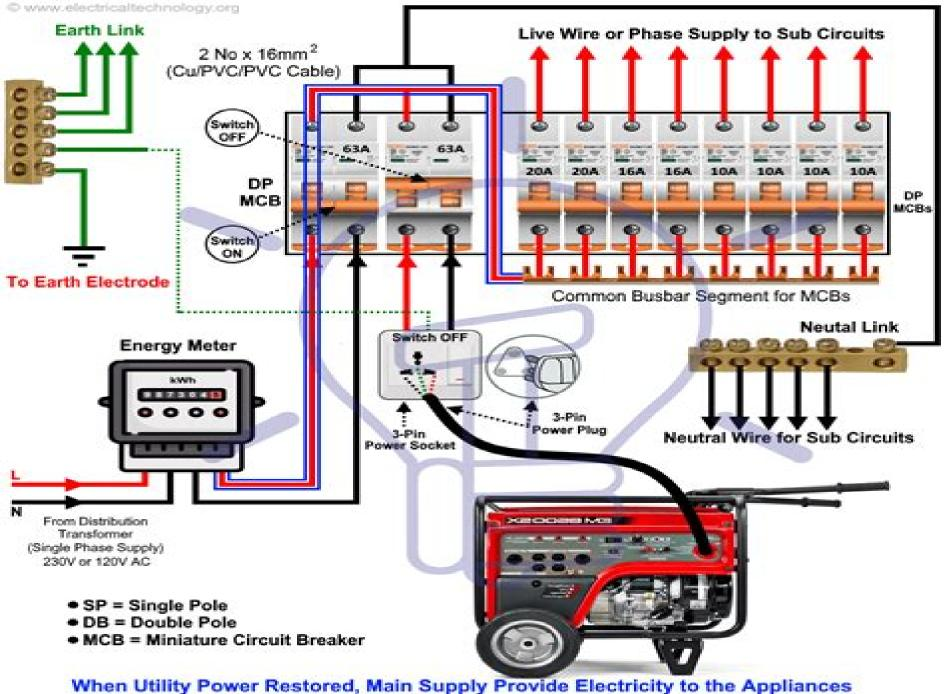
When Utility Power Restored, Main Supply Provide Electricity to the Appliance and Generator Remains Standby. The Blue Line Show the Power Flow Route
