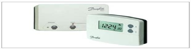
The TP5000 Si is a microprocessor based programmable room thermostat with many advanced features. The range includes battery powered hard-wired models and battery powered wireless versions. All models in the range utilise an advanced PI algorithm to provide close and accurate temperature control to reduce energy waste and ensure comfort under all load conditions.
