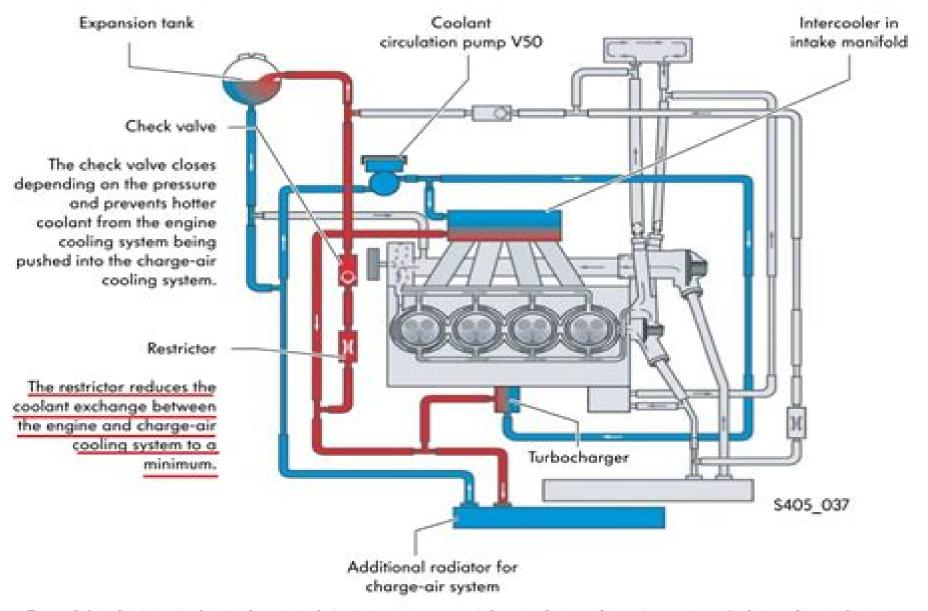
To cool the charge air, the coolant circulation pump is operated according to the requirements. It draws the coolant from the additional radiator at the front end and pumps it to the intercooler and to the turbocharger. The temperature difference between the air after the intercooler and the outside temperature is around 20°C to 25°C with high load requirements.
