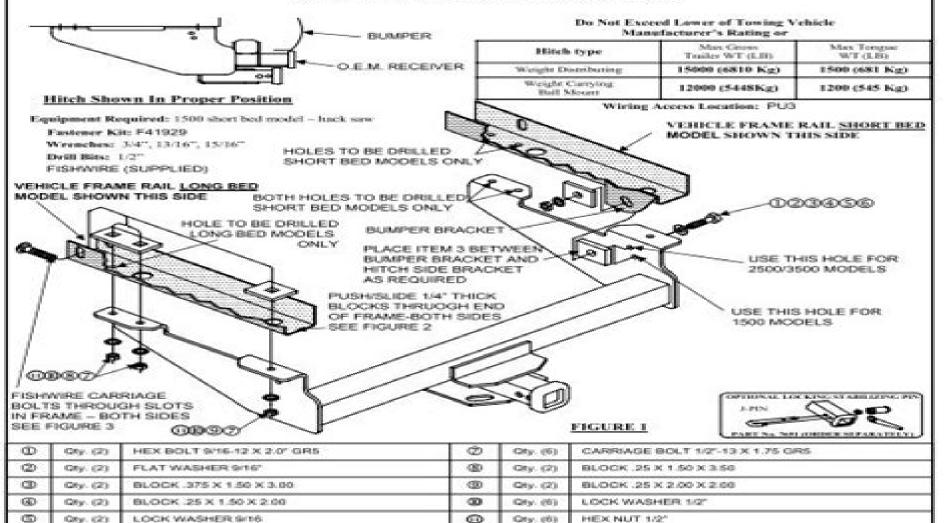
Tighten all 1/2-13 fasteners with torque wrench to 75 Lb.-Ft. (102 n\*m) Tighten all 9/16-12 fasteners with torque wrench to 110 Lb.-Ft. (149 n\*m)
